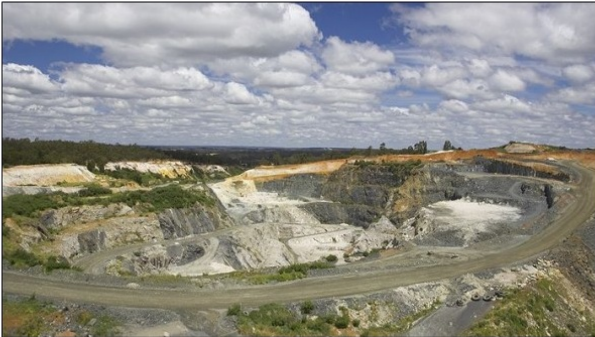
An area of the Greenbushes Lithium Mine in Australia. Note the telltale milky white areas indicative of this low iron, high technical grade ore.
