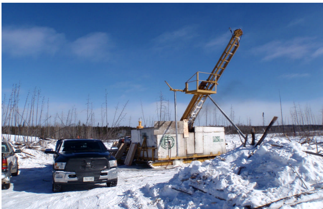
A drill rig in operation during the Phase I drilling program at PAK. Typically, the company takes advantage of a maintained winter road and the firm ground of winter time to move drill rigs in and out of the Project area.
